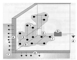
1) electrodes in walls and floor 2) connecting wires
